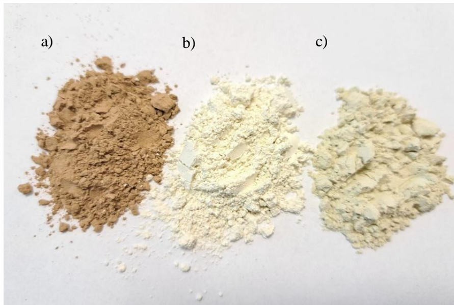
Fig. 1. Fuel additives used in powder form: a) halloysite; b) kaolin; c) bentonite.
