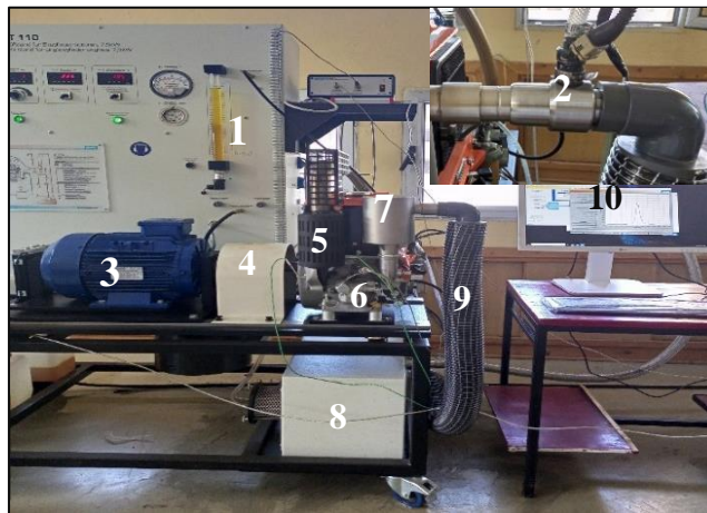
Fig. 1. The engine test rig setup, 1 – Fuel measuring tube, 2 – PFI(RCCI Engine), 3 – Dynamometer, 4 – Motor engine coupler, 5 – Exhaust manifold, 6 – Engine, 7 – Reactor, 8 – Air settling tank, 9 – Intake manifold, 10 - Computers for DAQ.
