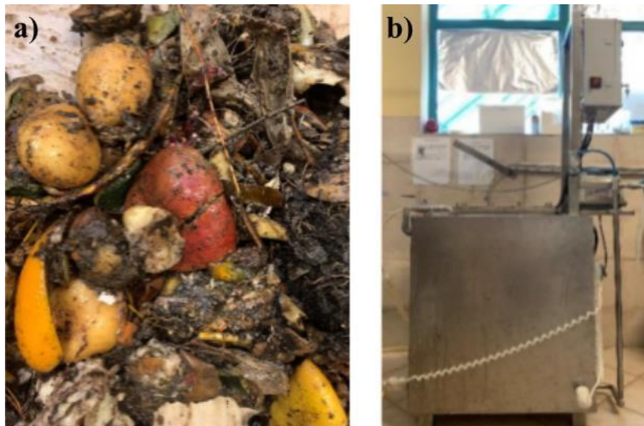
Fig. 2. A) Real biowaste after separation; b) The 100 L bioreactor used for the experiment
