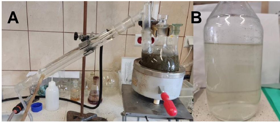
Fig. 4. Set for atmospheric distillation with cut silver fir needles (A) and its hydrosol (B)
